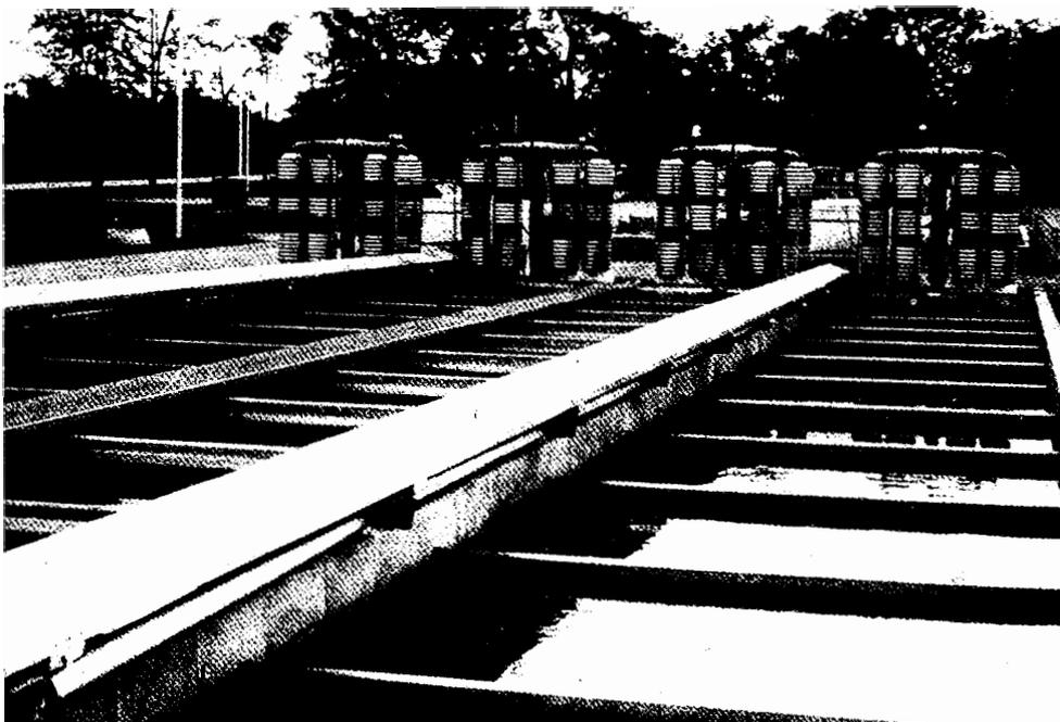
Packed columns used to aerate the water entering the raceways at the Wolf Lake Hatchery.
