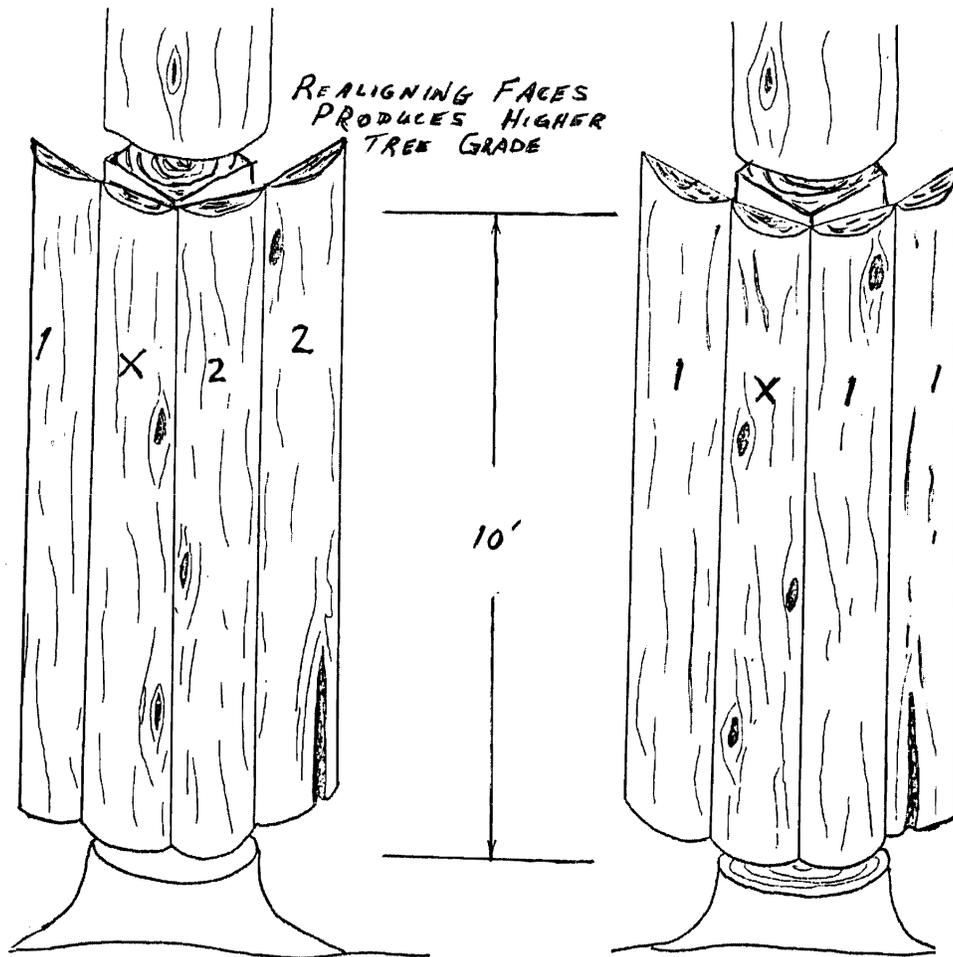
**Figure 19 - Realign Faces to Produce Higher Grades**
