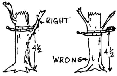
Figure 1 - Proper Technique for Measuring DBH with a D-Tape
