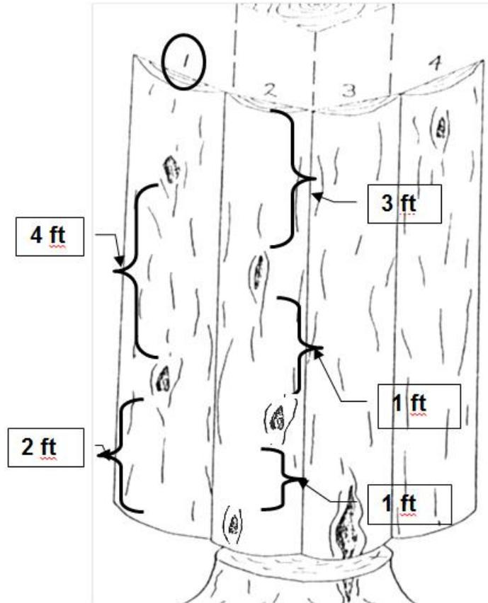
**Figure 18 - Identify the 3rd Best Face (Face 1) Which Must Have at Least Two, 2 Feet Clear Cuttings**
